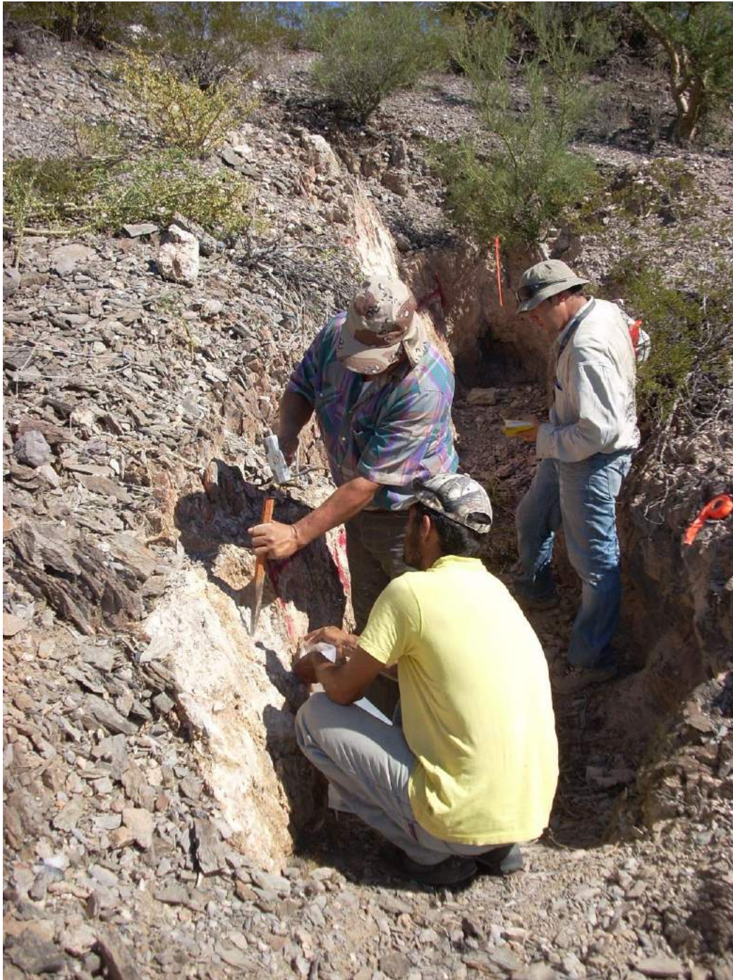
Photo 1. View northeast of trench along Mine Workings Shear Zone at Waypoints 206-207. Rock-chip samples ELZB 40-42 collected here ran 26.1 ppm, 8.8 ppm, and 19.3 ppm Au, respectively.
